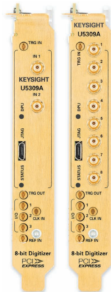
Figure 3. 2 and 8 channels U5309A front panels with analog inputs and multiple I/O signals.
